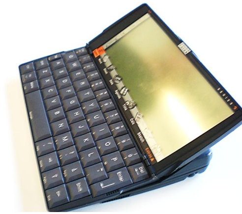
Figure 9.9. The Psion Series 5 handheld device, circa 1995. The resistive touch screen supports stylus or touch input. Note the counterweight on the bottom part of the clamshell that prevents the device from tipping over when one interacts with the screen.
